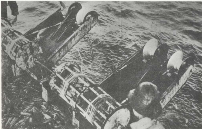
(Above) Squid jigging devices mounted on the rail of a boat, being operated by a hand crank.
